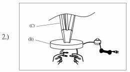
Step.2: Wire fixture to wires in outlet box. Install Green wire to Ground Screw.
