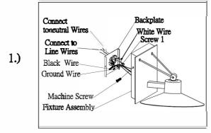
**Step 1:** Remove mounting bracket from fixture and install it to the electrical box. Wire fixture to wires in outlet box. Green wire is for ground
